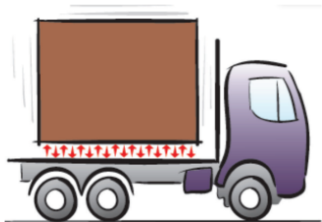
Figure 3: Vertical vibration during driving
