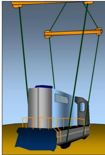
Arrangement with inward inclined secondary slings, estimated parameters
