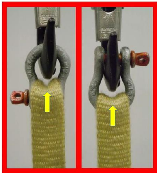
Folding, bunching, or pinching of synthetic slings
