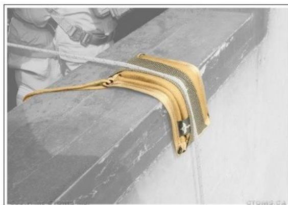
An unprotected rope can become damaged and unsafe when sawed over a rough or sharpe edge.
