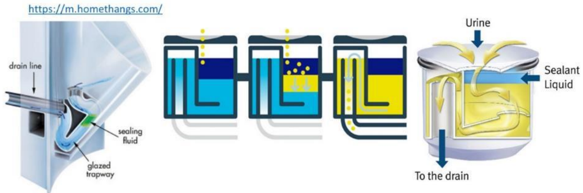
The Buoyant Sealant Maintains An Air-Tight Layer
