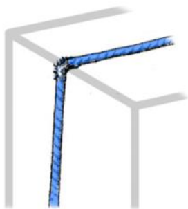
An unprotected rope can become damaged and unsafe when sawed over a rough or sharpe edge.
