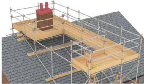
Chimney stack scaffolds (ridge, gable end and eaves chimneys)
